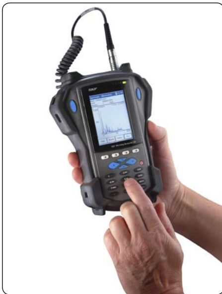
Condition monitoring per i mandrini
