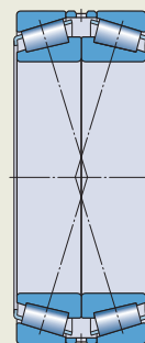
Matched bearings arranged face-to-face
