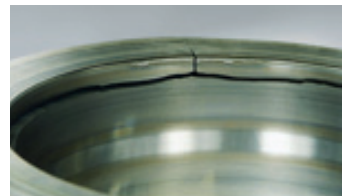
Figure 13 Thermal cracking is caused by high frictional heating due to sliding motion.
