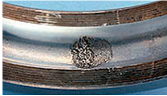
Figure 7 Electrical pitting are small burns created by arcs from improper electric grounding while the bearing is stationary.
