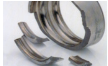
Figure 12 Forced fracture caused by a direct hammer blow.
