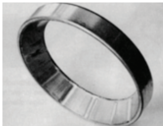
Figure 9 Plastic deformation appearance on the raceway after overloading.
