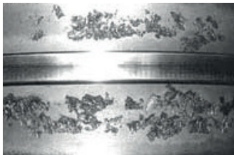
Figure 1 Fatigue spalling on the raceway
