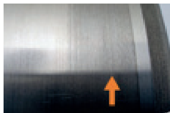
Figure 2 Adhesion occurs in equipment operating in the mixed and boundary lubrication regimes due to insufficient lube supply, inadequate viscosity, incorrect internal clearances, incorrect installation or misalignment.
