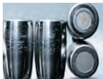
Figure 3 Abrasive wear is the result of inadequate lubrication or the ingress of foreign particles.
