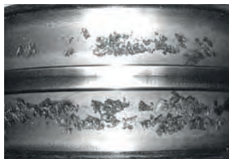
Figure 1 Fatigue spalling on the raceway
