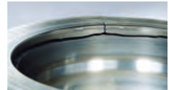
Figure 13 Thermal cracking is caused by high frictional heating due to sliding motion.
